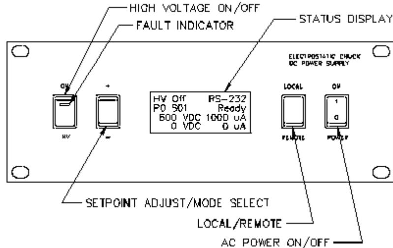
**Figure 3.1 - EPS200 Front Panel**
