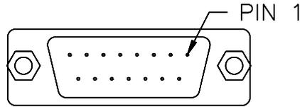
**Figure D.1 - Remote Control Connector**
