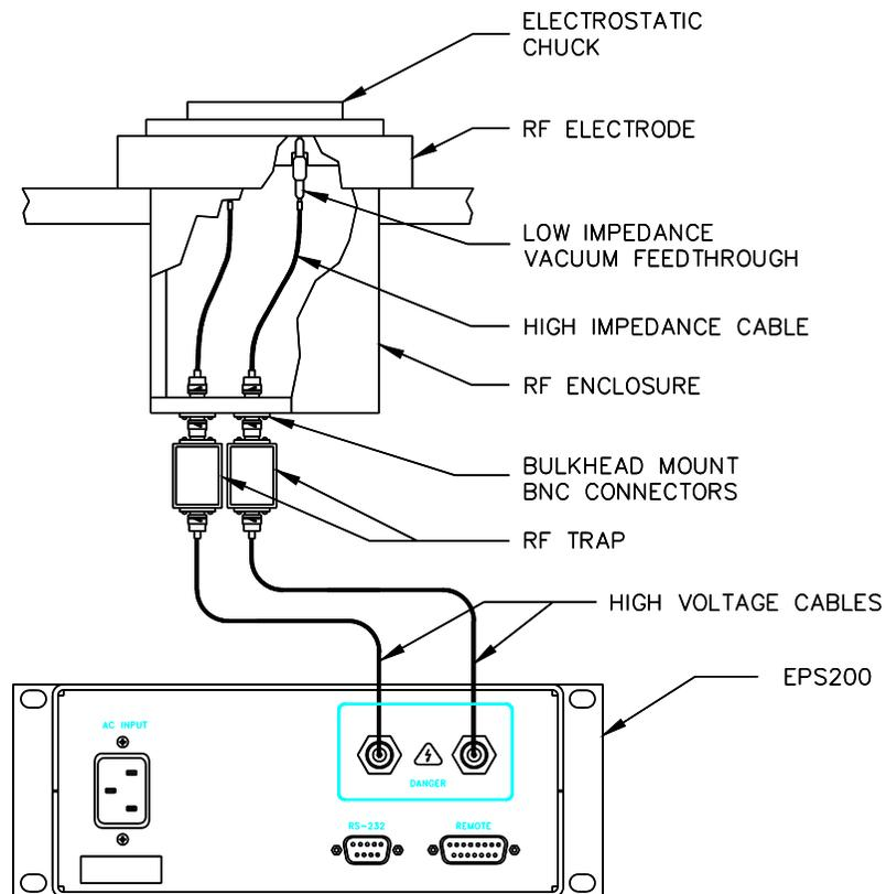
**Figure 2.2 - Typical Installation**
