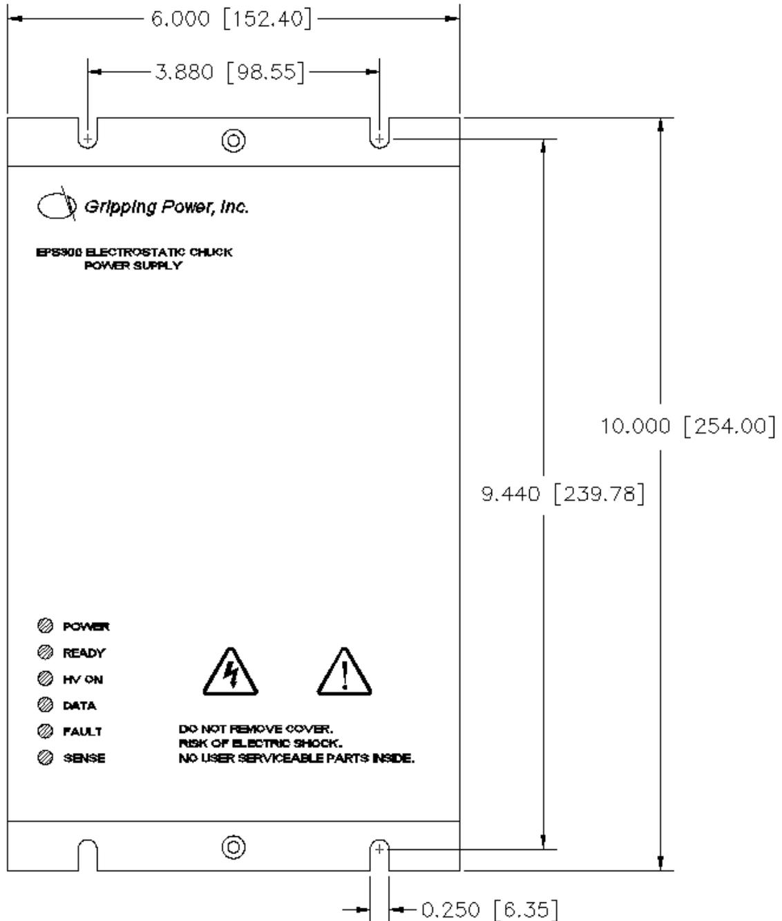
The unit can be mounted in any orientation, using four #8-32 or #10-32 screws and should be mounted as close to the electrostatic chuck as possible. Four mounting points are provided on the unit as shown.
